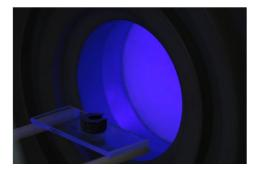
Because of the influence of the sample thrust in push-rod mechanical dilatometer made with high margin of error of linear expansion measurements. Fewer errors can be made with OD-201 optical dilatometer through as physical non- contact.
