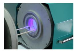
The biggest advantage compared to traditional mechanical push-rod dilatometers, is to provide the opportunity to measure directly without any physical contact with the sample.
